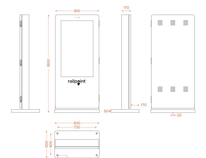
LCD panel: active matrix TFT LCD Display Glass: anti-reflective / anti-glare coated Internal media player housing Internal power output for power feed to media player Built-in option to add external WiFi aerial antenna Remote control support for full OSD features Front opening for maintenance. Three Year parts warranty
