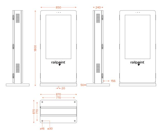
LCD panel: active matrix TFT LCD Display
